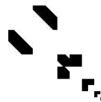
Figure 2.8. NS-form representation of the operator e^{\nu \Delta t \mathcal{L}} used in (2.4.20). Entries of absolute value greater than 10^{-8} are shown in black. The wavelet basis is Daubechies with M = 6 vanishing moments ( L_f = 18 ), the number of scales is n = 9 and J = 7 . We have set \nu = 1.0 and \Delta t = \Delta x = 2^{-9} .
