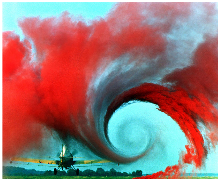
Figure 1: A NASA study on wingtip vortices qualitatively illustrates the wake turbulence
