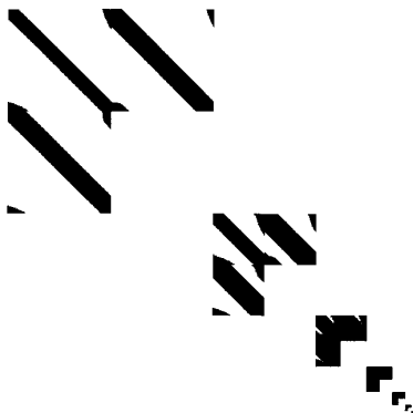
FIG. 13. The NS-form of LU factors for Example 2. The factors are combined together as \hat{T}_0 & \tilde{T}_0 and entries above the threshold 10^{-10} are shown in black.
