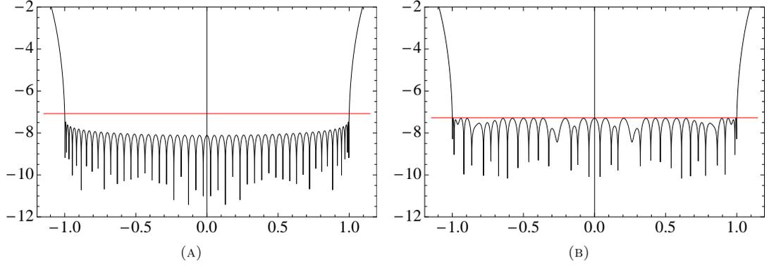
FIGURE 6.1. Logarithm of the error of the 24 node quadrature for bandlimit  $c = 50$ . In (a) we use nodes and weights from [24] and in (b) nodes from [24] and weights generated via  $\ell^\infty$  minimization. The horizontal lines at  $8.30 \cdot 10^{-8}$  in (a) and at  $5.26 \cdot 10^{-8}$  in (b) indicate the maximum  $\ell^\infty$  error within the bandwidth.
