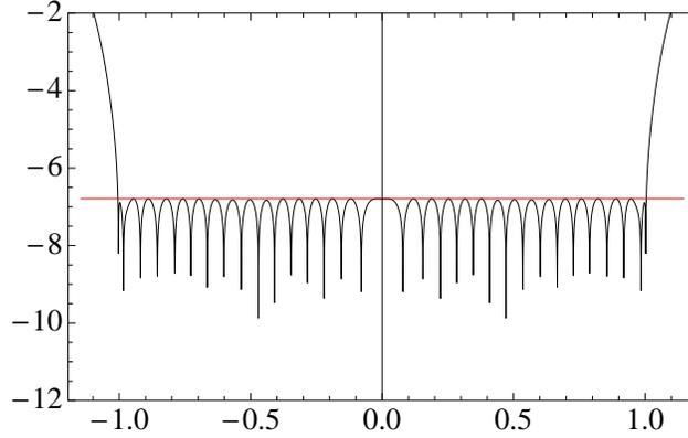
FIGURE 6.4. Logarithm of the error of the 24 node quadrature for bandlimit  $c = 50$  with weights generated by minimizing an  $\ell^2$  residual with an  $\ell^\infty$  constraint. Although the error has a near perfect behavior, the maximum absolute error  $1.62 \cdot 10^{-7}$  is worse than in Figures (6.1), (6.2) and (6.3).
