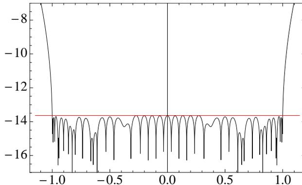
FIGURE 5.1. The logarithm of the error of the quadrature with 22 nodes ( $c = 10\pi$ ) for the weight function (5.2). The quadrature weights were generated via  $\ell^\infty$  minimization. The horizontal line at  $2.32 \cdot 10^{-14}$  indicates the maximum  $\ell^\infty$  error within the bandwidth.
