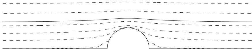
FIGURE 19. Streamline plot for the  $\alpha = .48, \omega = 1$  perturbation of potential flow.
