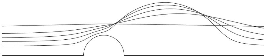
FIGURE 17. Vortex tubes, with  $\omega = 1$ , perturbations of a vortex in Figure 3. Values of  $\alpha$  are .1, .2, .3, .4 and .5.
