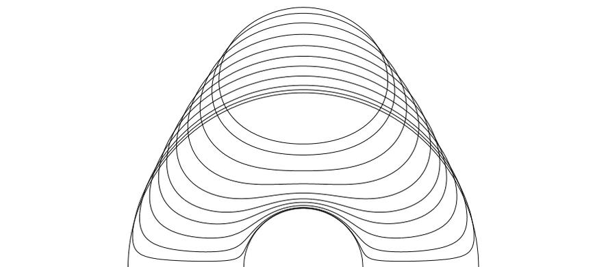
FIGURE 11. Vortex rings perturbed off the concentric spherical attached vortex, with  $\kappa = 15$ . Values of  $\alpha$  are 0, -.005, -.03, -.1, -.22, -.36, -.6, -1, -1.6, -2.4, -3.
