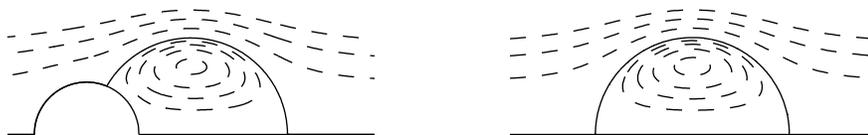
FIGURE 2. On the left is a streamline plot for flow past a sphere with an attached vortex with  $M = 4$ ,  $\omega = 2.2$ . On the right is a streamline plot for Hill's spherical vortex of radius 1.85, which has the same value of  $\omega$ .
