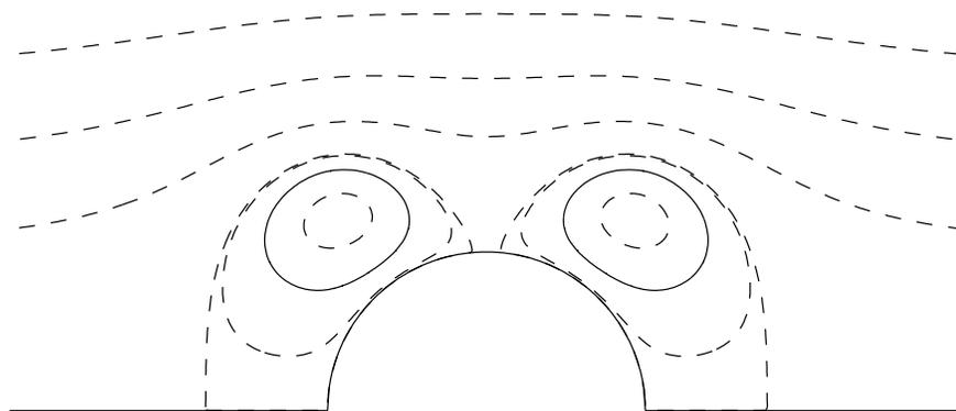
FIGURE 14. Streamline plot for flow with  $\kappa = 8$  with vortex regions near the end of the family shown in Figure 13. The stagnation points are near the top of the circle.
