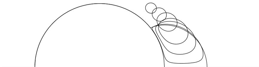
FIGURE 8. Vortex rings trailing the sphere, with  $\kappa = 2$ . Values of  $\alpha$  are 0, -.002, -.02, -.06, -.14, -.22, -.30 .
