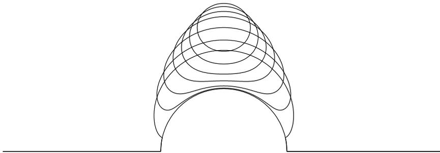
FIGURE 12. Vortex rings perturbed off an attached vortex band,  $\kappa = 7$ . Values of  $\alpha$  are 0, -.02, -.1, -.3, -.58, -1, -1.58.
