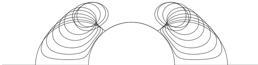
FIGURE 13. Vortex ring pairs, with  $\kappa = 8$ . Values of  $\alpha$  go from 0 to  $-.43$ , then increase again to  $-.27$  as the vortex regions move toward the vertical axis.
