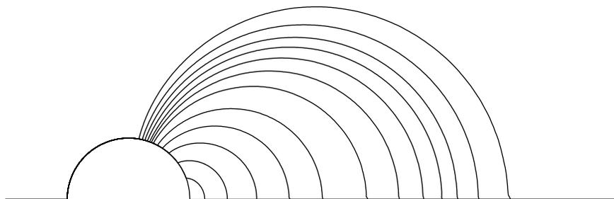
FIGURE 3. Attached ( $\alpha = 0$ ) trailing vortices. Values of  $M$  are .01, .1, .4, 1, 2, 4, 6, 8, 10, 12, 15 and 20.
