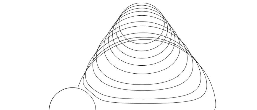
FIGURE 10. Vortex rings trailing the sphere, with  $\kappa = 15$ . Values of  $\alpha$  are 0, -.08, -.2, -.6, -1.98, -2.97, -3.98, -5.17 and -6.51.
