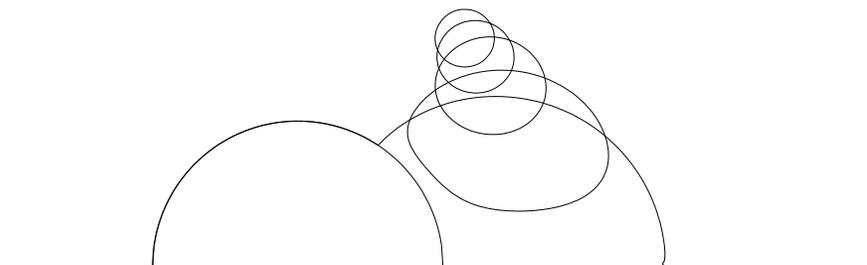
FIGURE 9. Vortex rings trailing the sphere, with  $\kappa = 5$ . Values of  $\alpha$  are 0, -.1, -.59, -1.04 and -1.43
