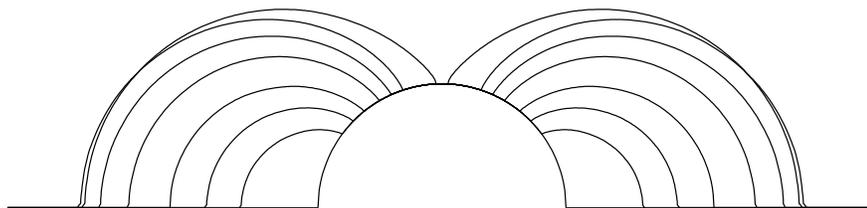
FIGURE 5. Solutions with two symmetric attached vortex regions. Values of  $M$  are .2, .5, 1, 2, 3, 4, 4.65.
