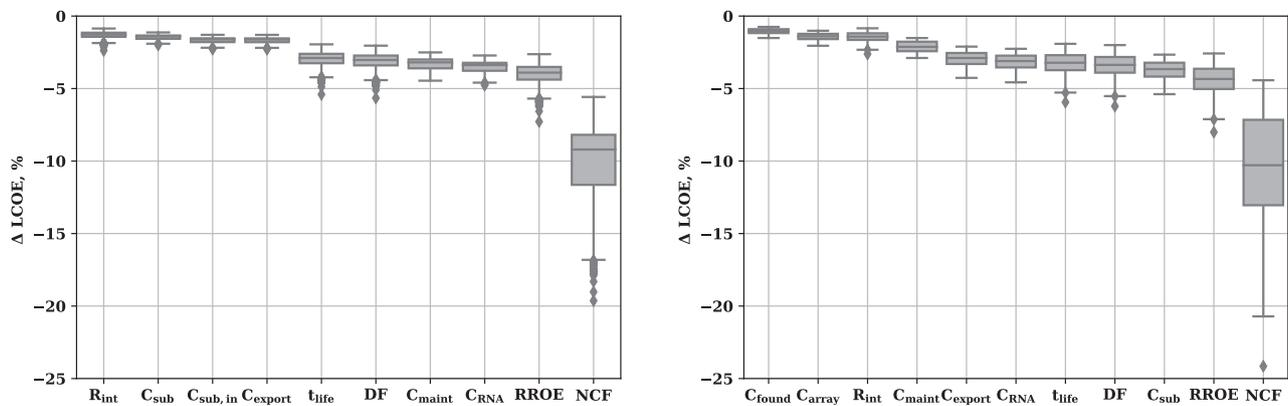
Fig. 3. Spatial variability in LCOE attributed to technological and financial innovations for fixed-bottom (left) and floating substructures (right) in the United States. Input variables that produce  $\Delta\text{LCOE} < 1\%$  are not shown. The average LCOE for fixed-bottom and floating substructures across all U.S. sites considered is \$152/MWh and \$191/MWh, respectively.
