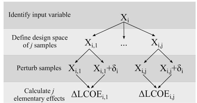
**Fig. 2.** Process for calculating the mean elementary effect for an ORCA input variable.
