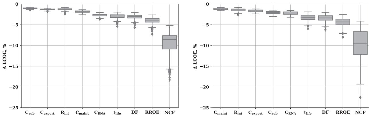
Fig. 6. Sensitivities of LCOE to cost and financial categories using constant perturbations of  $\delta = 10\%$  for fixed-bottom (left) and floating (right) substructures in the United States. Input variables that produce  $\Delta LCOE < 1\%$  are not shown. The average LCOE for fixed-bottom and floating substructures across all U.S. sites considered is \$152/MWh and \$191/MWh, respectively.
