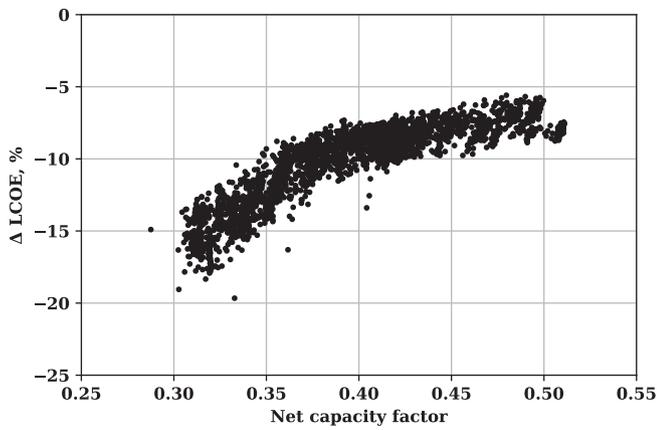
Fig. 4. Spatial variability in LCOE compared with net capacity factor for fixed-bottom substructures at all sites in the United States.
