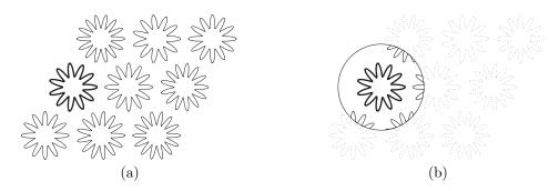
Fig. 2. In order to determine the  $R^{(i)}$  and  $L^{(i)}$  that compress the interaction between  $\Gamma_i$  (shown in bold) and the remaining contours, it is sufficient to consider only the interactions between the contours drawn with a solid line in (b).
