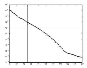
Fig. 6. Plot of the singular values of  $X^{(i)} = [H^{(i)} | (V^{(i)})^*]$  where  $H^{(i)}$  and  $V^{(i)}$  are as in Figure 5. The numerical rank of  $X^{(i)}$  is approximately 80, which is larger than the individual ranks of  $H^{(i)}$  and  $V^{(i)}$ .
