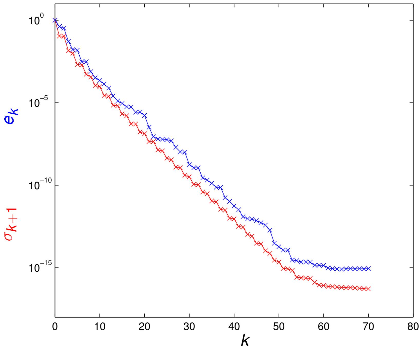
The red line indicates the singular values  $\sigma_{k+1}$  of  $\mathbf{A}$ . These indicate the theoretically minimal approximation error.
