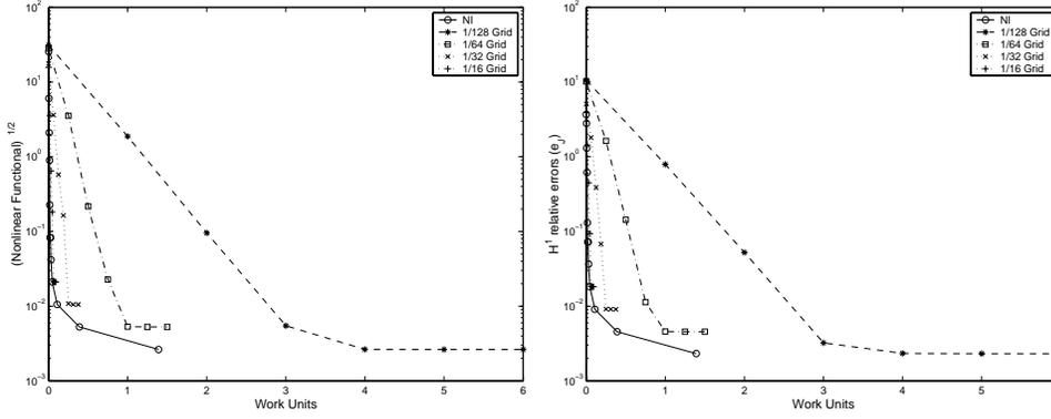
FIG. 4.3. *First-stage functional. Functional and  $H^1$  error measures for standard Newton iterations and NI with imposed boundary conditions. One work unit is the equivalent of one step on the  $h = \frac{1}{128}$  grid using 2  $V(1,1)$ -cycles.*
