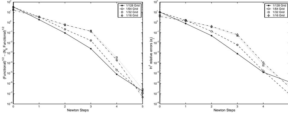
FIG. 4.4. Newton convergence, using standard Newton iterations with imposed boundary conditions, in both functional and  $H^1$  error measures. Difference between the value at the current and sixth Newton steps are plotted.
