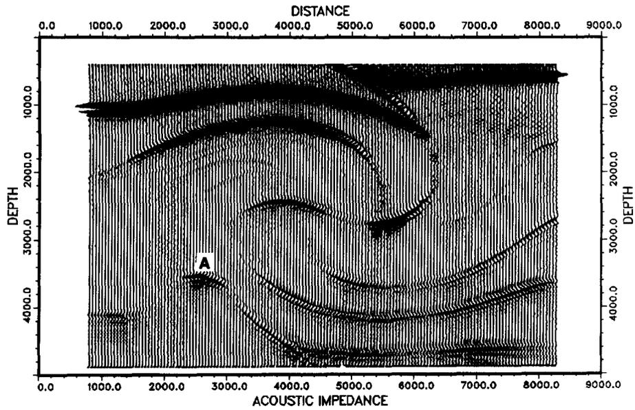
Fig. 7. Reconstruction of the acoustic impedance.
