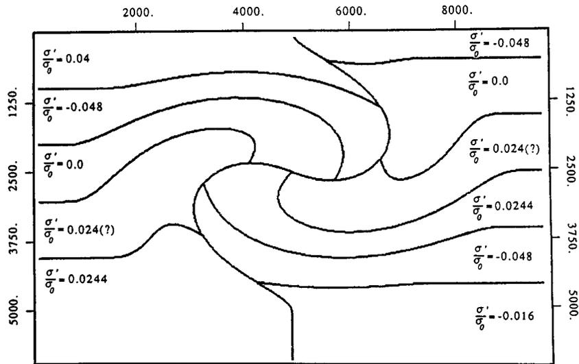
Fig. 3. The specific volume model showing relative perturbation with respect to the background medium.
